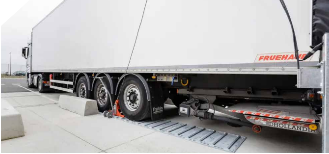
The truck restraint system POWERCHOCK 7 is locked on the restraining plate that is anchored to the ground.
