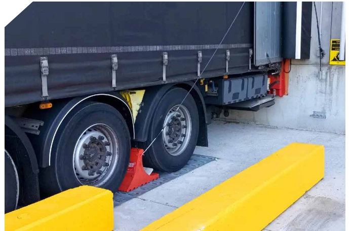
Vehicle secured with at the loading dock with the portable wheel chocking system POWERCHOCK 3.
